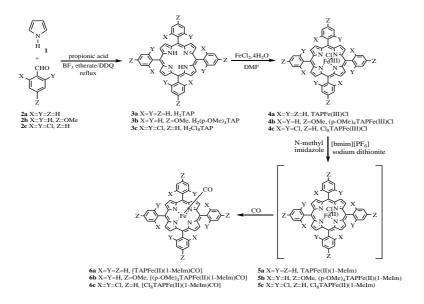
Scheme 1: Binding of different aryl substituted meso-tetraarylporphyrins with CO inionic liquid.
